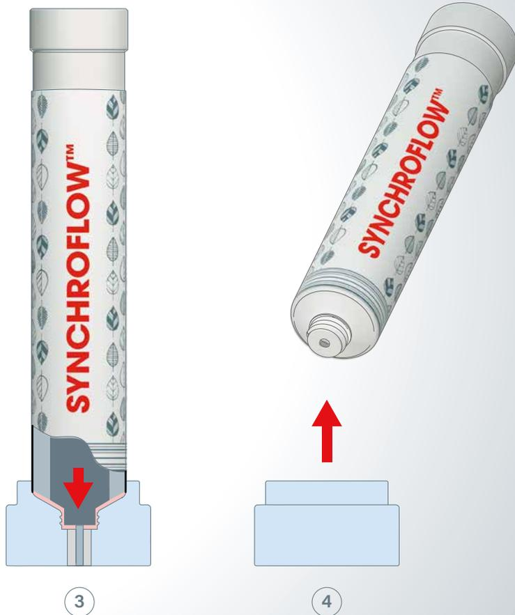
③ Inner part (F) of the mandrel is pushed further down to form the mold for the tube head. ④ The mandrel lifts up, the shoulder is perfectly moulded and welded with a clean orifice to the sleeve.
