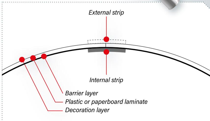
To prevent the paperboard from absorbing external moisture, a second strip is welded on the outside of the sleeve.
